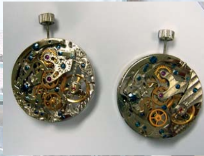
A skeletonized and decorated movement for Naked Watch
